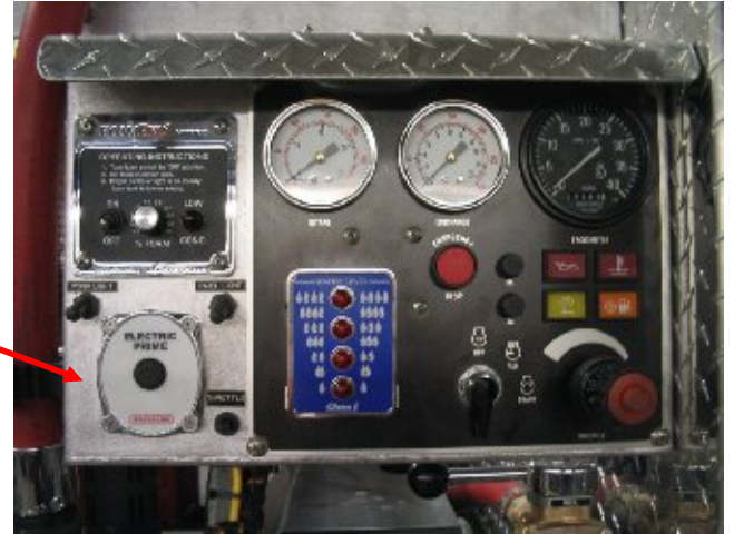
PUMP OPERATOR CONTROL PANEL
