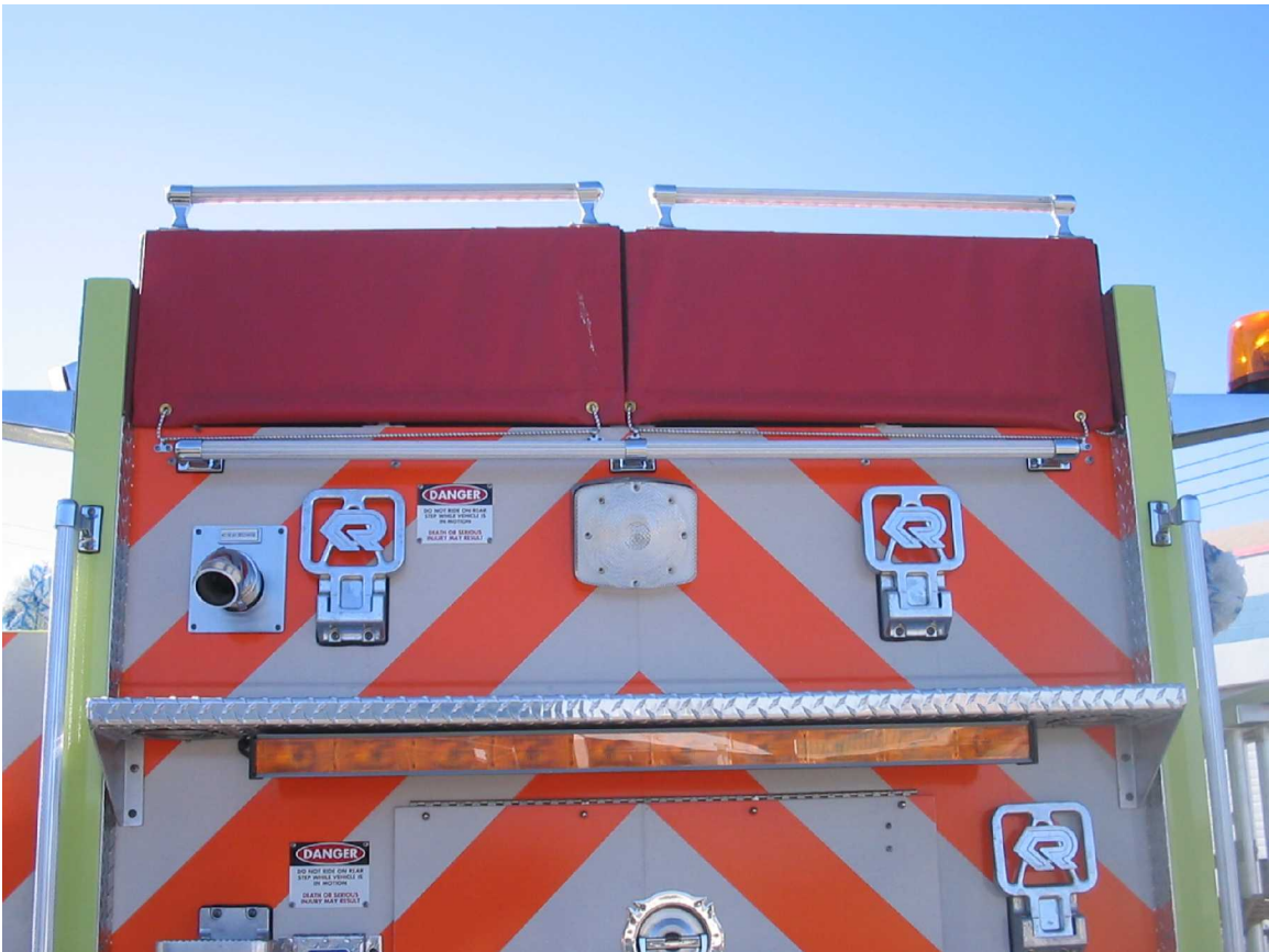
2-2 1/2" QUICK FILLS, 10 X 10 QUICK DUMP, FOLDING TANK STORAGE & REAR WATER LEVEL INDICATOR REAR TRAFFIC ADVISOR WITH FULL WIDTH REAR INTERMEDIATE HOSEBED ACCESS STEP MAIN HOSEBED HINGED ALUMINUM COVER & VINYL END FLAPS WITH HANDRAILS & FOLDING STEPS
