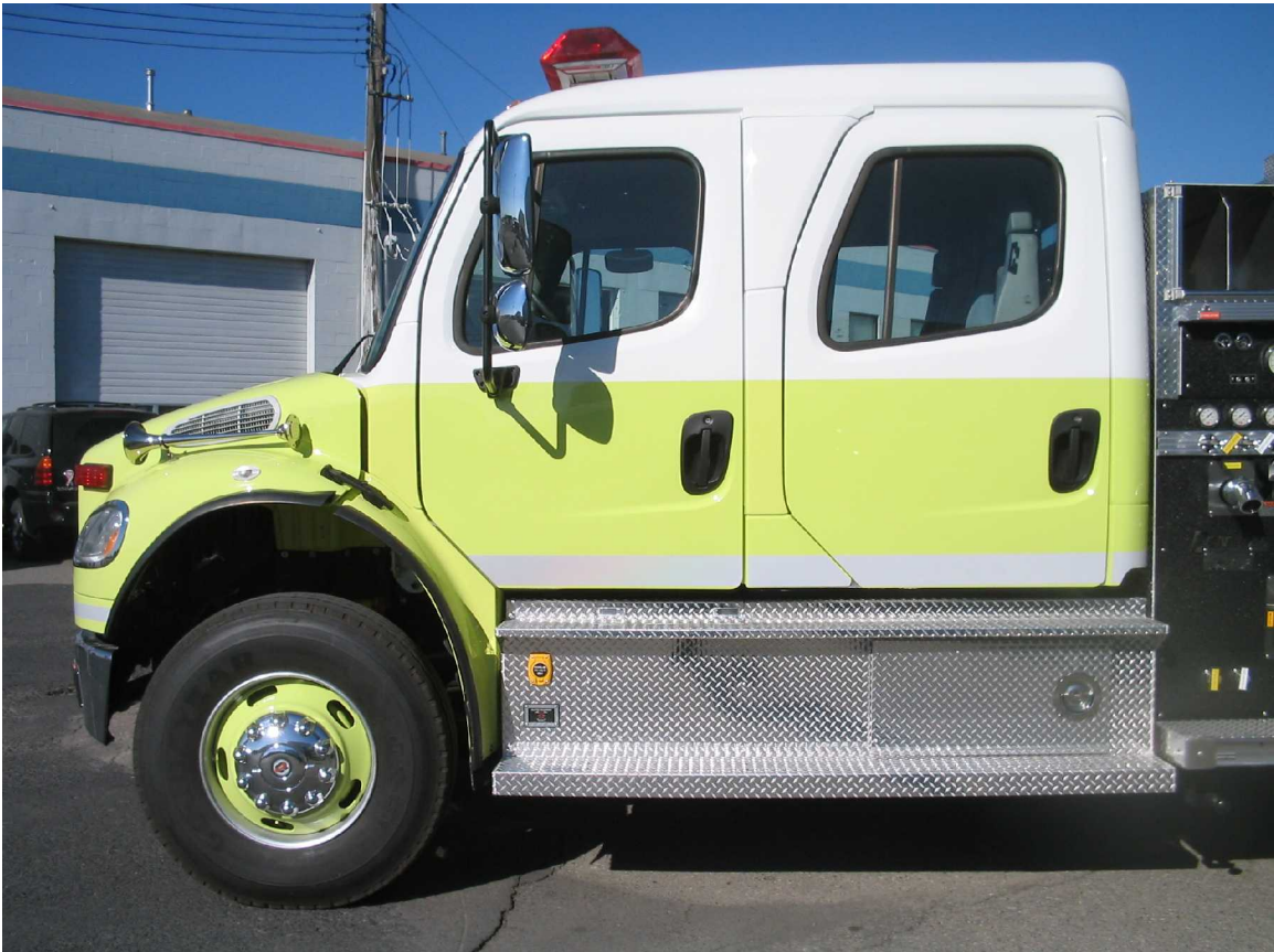
FREIGHTLINER M-2 4 DOOR CHASSIS WITH 315 HP CUMMINS DIESEL ENGINE & AUTOMATIC TRANSMISSION CHROME FRONT BUMPER WITH RECESSED ELECTRONIC SPEAKER, CODE 3 LED FRONT EMERGENCY LIGHTING KUSSMAUL AUTO EJECTOR WITH BATTERY & CHASSIS AIR CONDITIONER LARGE UNDER CREW CAB STORAGE COMPARTMENT & ALUMINUM CAB ACCESS STEP OVER LAID
