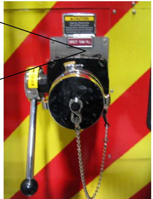
TWO 2 1/2" DIRECT TANK FILLS REAR MOUNTED
