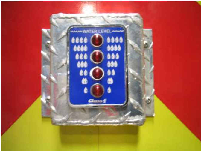
REAR MOUNTED WATER LEVEL GAUGE
