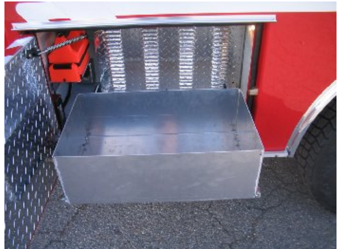
Slide out storage trays in lower rear compartment
