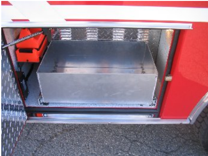
Slide out storage trays in lower rear compartment
