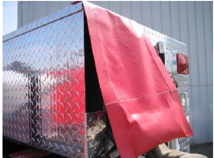
Under body enclosed Lightweight suction hose storage
