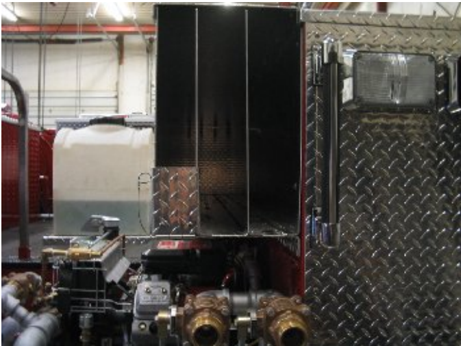
Akron gated discharges and suction inlets
