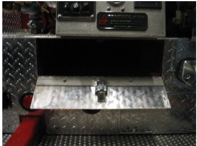
Under body enclosed Lightweight suction hose storage
