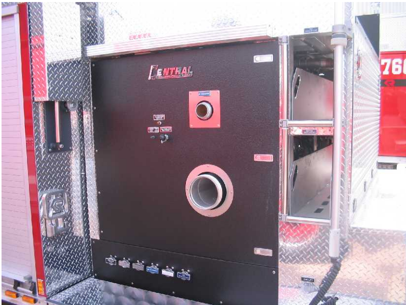
Closed Pump Access Door
