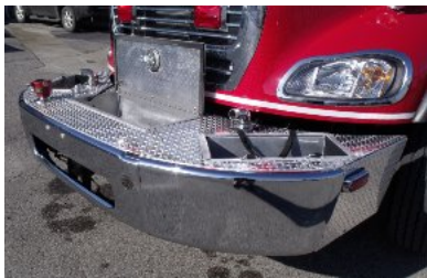
FRONT BUMPER DISCHARGE ROLLED 2 1/2" HOSE LAYS
